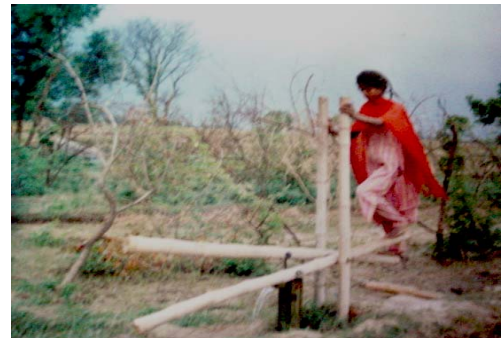
Treadle pump for irrigating vegetable farm
